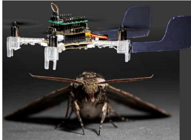
'Smellicopter' is the nickname for this autonomous drone that uses a live antenna from a moth (hawkmoth, the type depicted here) to navigate towards smells.
