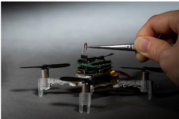
By adding tiny wires to either end of the antenna (the arc being attached here), the researchers were able to connect it to a circuit and record its responses to a puff of floral scent.
